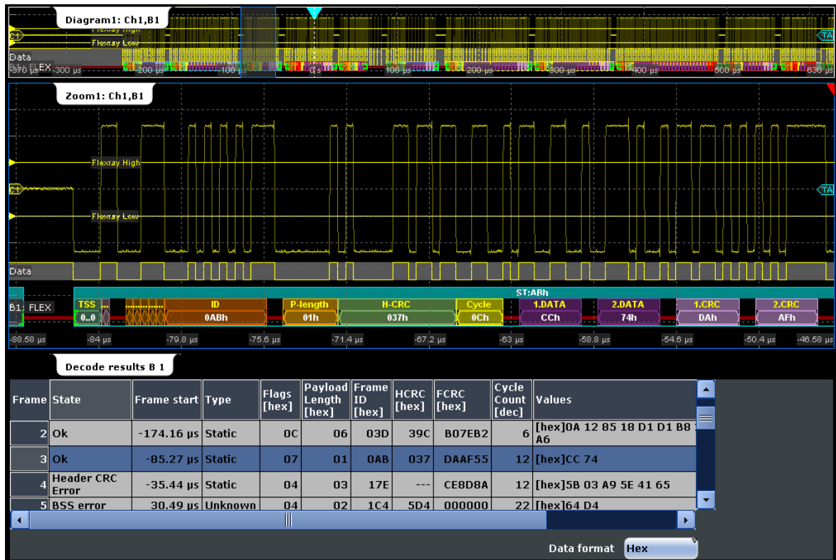
Fig. 10-16: FlexRay - decoded dynamic slot and results table
